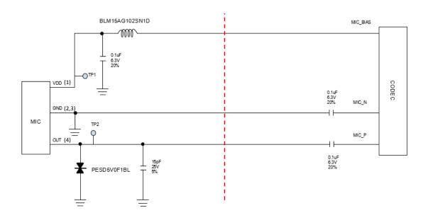
NOTE: It is recommended that the components on the left side of red line be placed close to MIC, and components on the right side of red line be placed close to codec.
